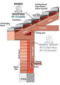
**LIGHT REFLECTIVITY -** Gains of up to 40% can be obtained by using Rhino Roofing RP-101 as an exposed internal roof lining. Efficiencies in lighting loads are also evident. Conforms to AS/ NZS 4859.1-2002.
